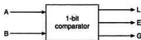
Block diagram of a 1-bit comparator.
